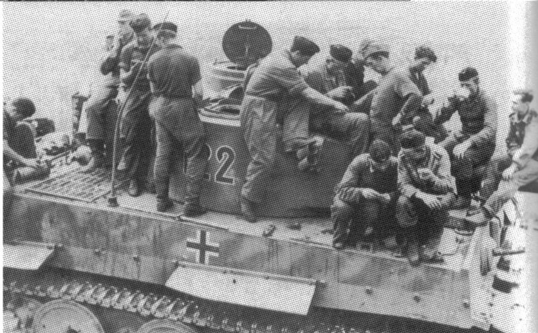
Two photographs of Tiger '122' from s.Pz.Abt.503 in the middle of August 1943. In the lower photo, the crew and mechanics are taking a break. The tank displays many signs of combat it has seen; missing mudguards and tools, a missing smoke candle discharger, a damaged roadwheel and a bent antenna. The missing mudguards also provide some insight on how the camouflage paint has been applied.
