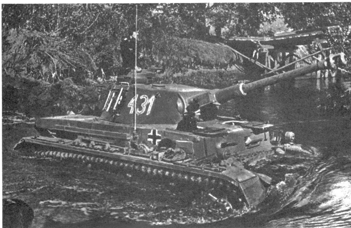
A Pz.Kpfw.III Ausf.N armed with the 7.5cm KwK L/24 gun that was being phased out on Pz.Kpfw.IV and StuG.III production. The new insignia of 7.Panzer-Division is also visible beside the driver's visor. Markings indicate it is the fourth (4) vehicle assigned to the Aufklärung Zug (1) in the Regimental Stabskompanie (R) which is unusual, as according to the table of organization, it should have been the third vehicle assigned to the Nachrichten Zug of the Battalion staff. Pz.Rgt.25 had 55 Pz.Kpfw.III on hand for Operation 'Citadel' on July 1, 1943, 12 of which were Pz.Kpfw.III Ausf.N.
