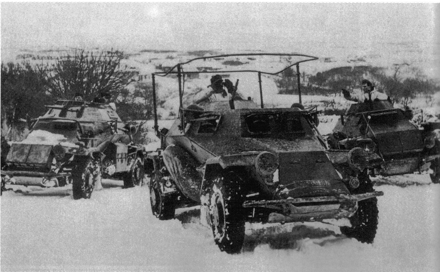
A trio of leichte Panzerspähwagen on a reconnaissance mission in the Don River area in the middle of February, 1943. From left to right, they are an Sd.Kfz.222, an Sd.Kfz.223 and an Sd.Kfz.221. Only the Sd.Kfz.222 has received any winter camouflage paint while the other two vehicles are still finished in their standard dark gray paint scheme.
