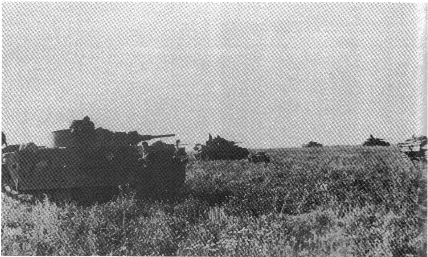
A Pz.Bef.Wg.III Ausf.J, fitted with the 5cm KwK L/42 and a full set of schürzen, photographed in the Bjelgorod area in late July 1943. It has also been uparmored with the additional 20mm spaced armor plate on the mantlet and, probably, on the front of the hull as well. Barely visible on the original print is the star antenna mounted on the rear of the engine deck. The white outline tactical number 'R02' indicates this vehicle is assigned to the Regimental Adjutant.
