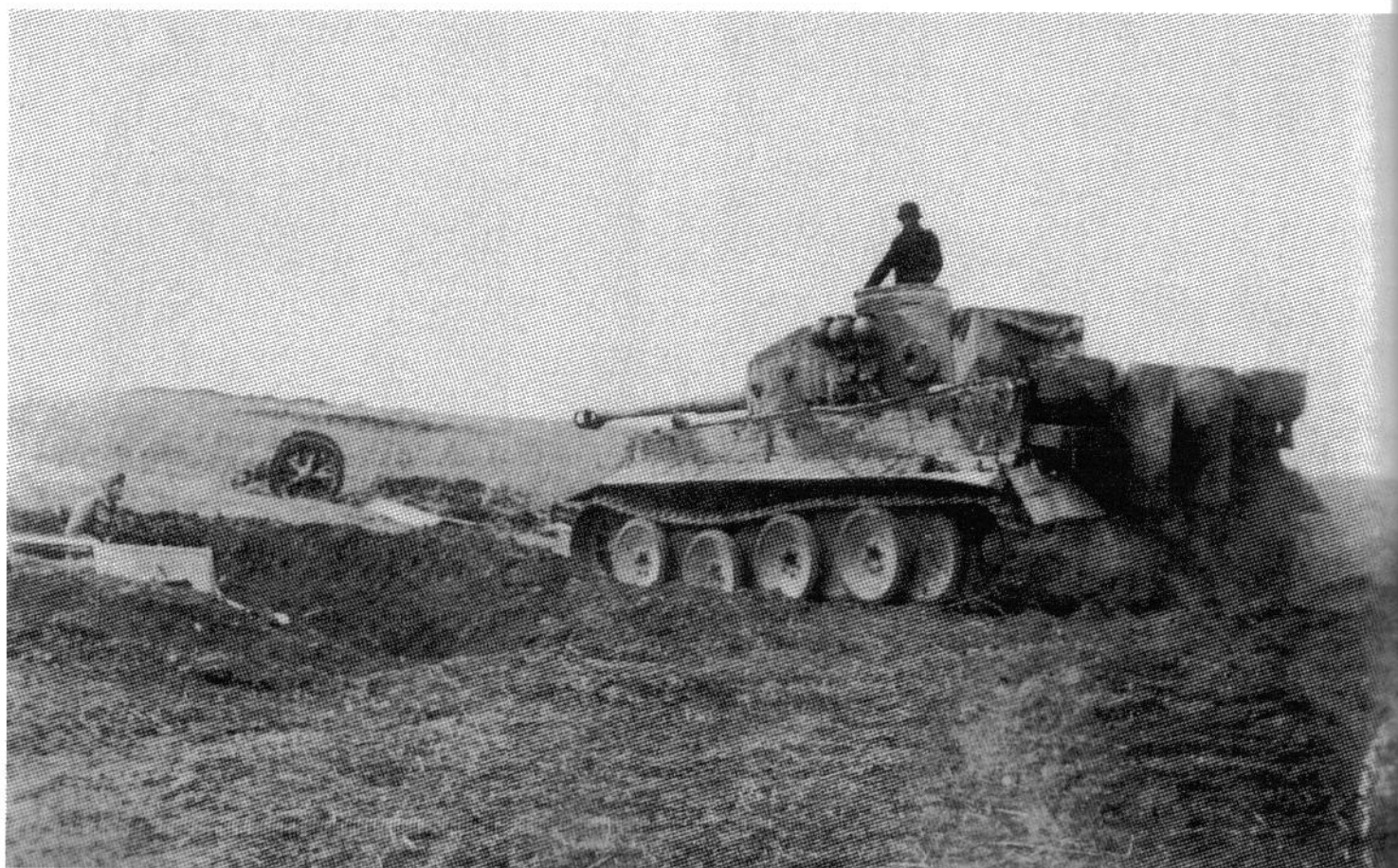
Two photos of Tigers employed by s.Pz.Abt.505 for Operation 'Citadel' in the northern sector during July 1943. Both vehicles are finished in the same way with a green or brown wavy camouflage pattern over the sand yellow base and barbed wire strung along the sides of the tank to discourage Soviet infantry from boarding. They are from the early production series, still with the Feifel air cleaners but without the turret mounted smoke candle dischargers that were discontinued in June 1943. White outline tactical numbers have been painted on the side of the turret.
