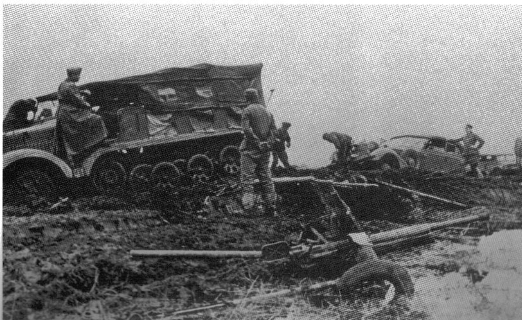
An Sd.Kfz.6 5-ton half-track prime mover being used to tow a staff car bearing a General's rank pennant. Normally, the rank pennant was carried on the right mudguard and the command pennant was carried on the left. When the rank pennant was on the left mudguard, this indicated the officer was not authorized to carry a command pennant. In the foreground is a Soviet 45mm Model 1932 anti-tank gun that has been abandoned by the retreating Russian Army.
