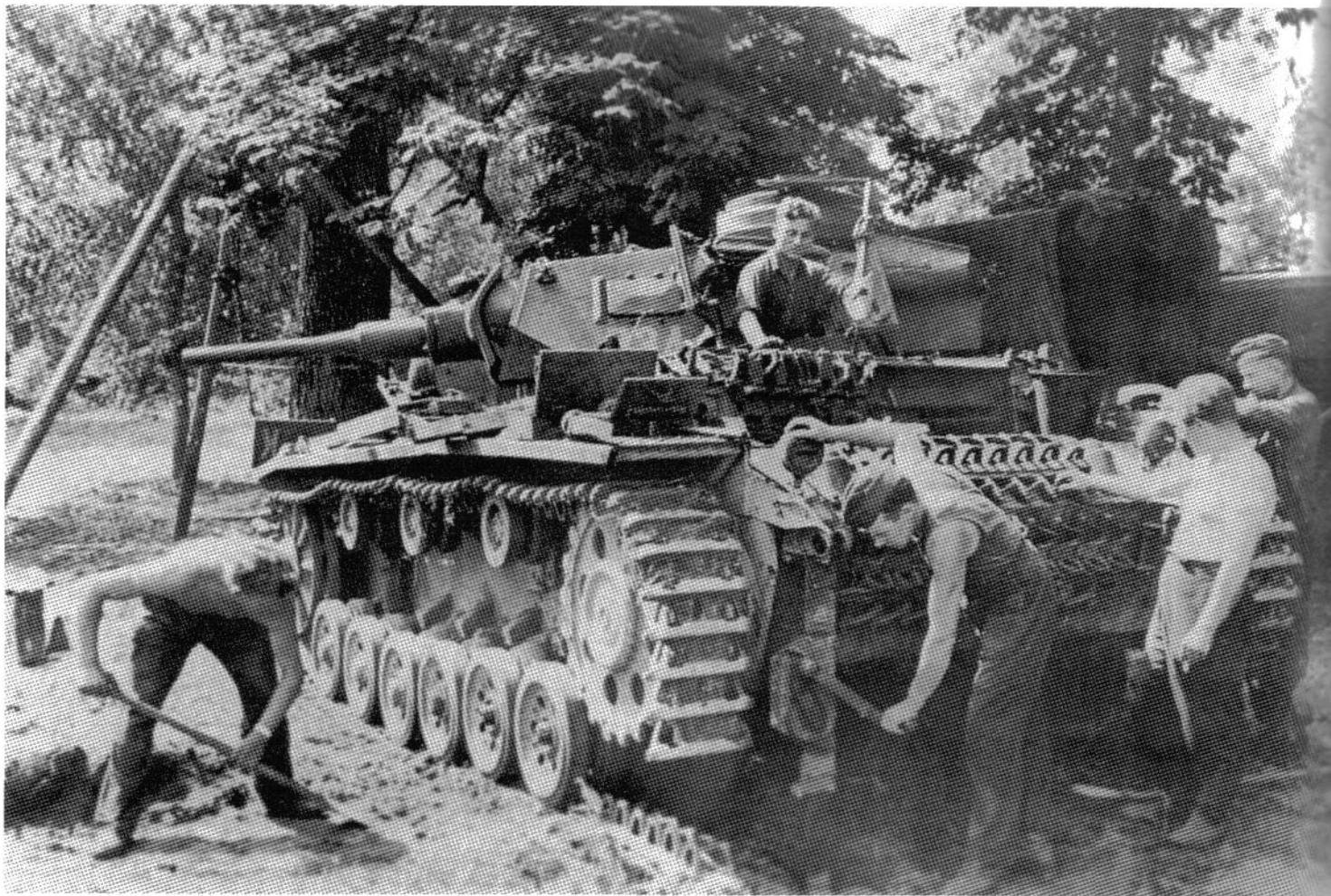
The crew of this Pz.Kpfw.III Ausf.F perform track maintenance during a lull in the fighting. It has been refitted with a 5cm KwK L/42, in place of its original 3.7cm KwK L/46.5 gun, along with a later cupola. The tactical number '334' appears on the sides of the turret in yellow along with a white letter 'K' on the rear mudguard. During July and August, at the height of the summer offensive in the central and southern part of the Eastern Front, the Germans lost 396 tanks of this type. During the same time, 462 replacements were produced.
