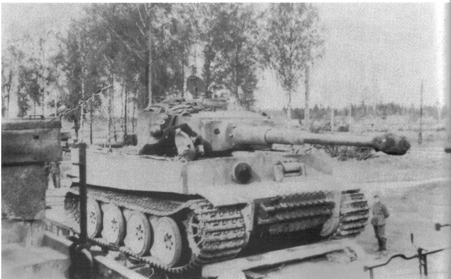
Two photographs of one of the first nine Tigers of s.Pz.Abt.502 being unloaded from a railroad flatcar at its destination in Russia in the late autumn of 1942. It was produced in early November 1942 as it is fitted with the new standard track but still has not been fitted with the side track guards. Not visible in the photos is the Pz.Kpfw.III stowage bin carried on the rear of the turret. The tactical number '102' has been painted in white outline on the side of the turret along with a large white outline Balkenkreuz on the side of the hull just ahead of the last outside roadwheel and the emblem of s.Pz.Abt.502, a white outline 'Mammut', on the front plate. Though it appears a light color, it is still in its original dark gray paint with a heavy coating of dust.
