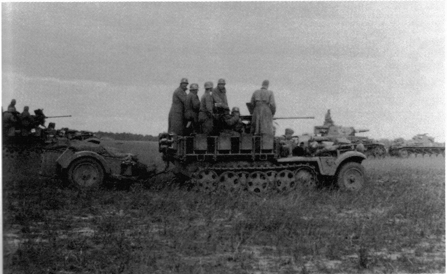
A pair of Sd.Kfz.10/4 half-tracks armed with 2cm FlaK38 anti-aircraft guns provide support to one of the Panzer-Divisions during their advance into Russia. With a crew of 7, space was at a premium, which can be easily seen here. In action, the sides of the gun platform could be folded down to provide additional space for the crew to maneuver around the gun. Magazines for the gun were carried in ready racks on the folding sides of the platform and usually, a single axle trailer was towed, carrying additional ammunition. A Pz.Kpfw.II and a Pz.Kpfw.IV Ausf.D can be seen in the background.
