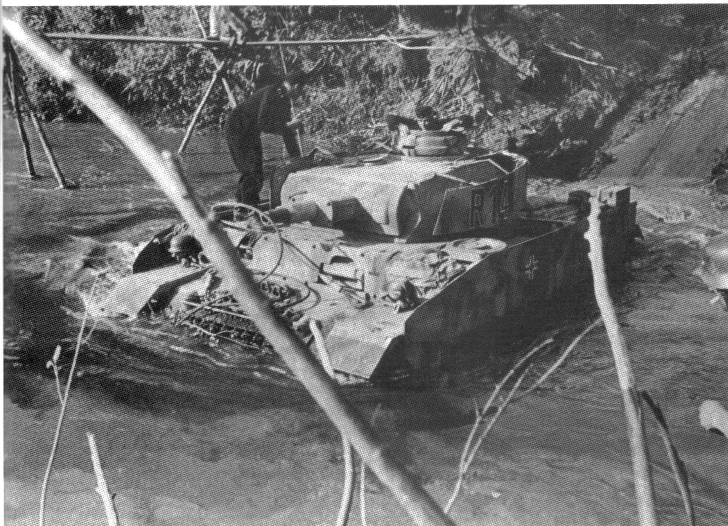
A Pz.Kpfw.III Ausf.N armed with the 7.5cm KwK L/24 gun that was being phased out on Pz.Kpfw.IV and StuG.III production. The new insignia of 7.Panzer-Division is also visible beside the driver's visor. Markings indicate it is the fourth (4) vehicle assigned to the Aufklärung Zug (1) in the Regimental Stabskompanie (R) which is unusual, as according to the table of organization, it should have been the third vehicle assigned to the Nachrichten Zug of the Battalion staff. Pz.Rgt.25 had 55 Pz.Kpfw.III on hand for Operation 'Citadel' on July 1, 1943, 12 of which were Pz.Kpfw.III Ausf.N.
