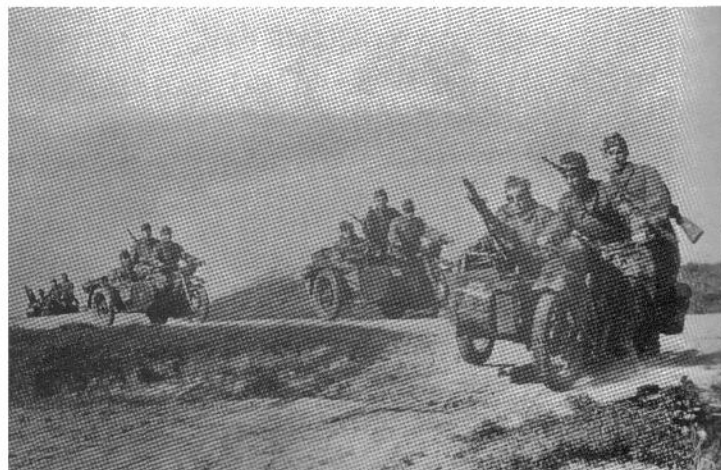
Kradschützen troops on BMW R12 combinations swing off a country road into a field in August 1943. The sidecar on the machine closest to the camera is fitted with an MG34 mount and appears to have suffered some damage to its front end. There is an illegible emblem painted on the front of each sidecar.
