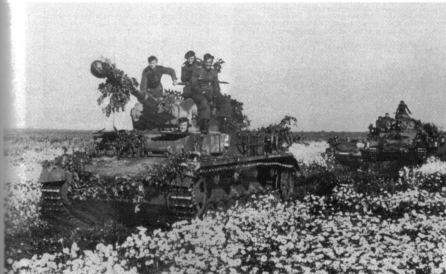
Two new Pz.Kpfw.IV Ausf.F2 of Panzer-Grenadier-Division 'Großdeutschland' march across the Russian steppes in the Don bend, August, 1942. They are painted in dark gray with sand colored spots sprayed on randomly and have foliage added to break up the shape of the vehicle. Armed with the 7.5cm KwK40 L/43, the Pz.Kpfw.IV Ausf.F2 finally gave the German Army superiority over the Russian KV-1 and T-34.
