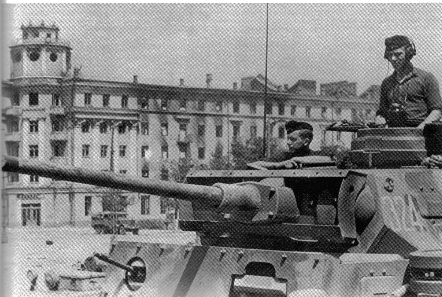
A closeup of a late Pz.Kpfw.III Ausf.J equipped with the 5cm KwK 39 L/60 gun, traveling through the city of Voronezh in late June or early July, 1942. It has been fitted with the 20mm spaced armor hull plate introduced on the Ausf.L and although the mounting plates on the mantlet have been installed, the 20mm plate is yet to be fitted here. The vehicle is finished in dusty coat of dark gray with a camouflage pattern of large, green irregular spots. The tactical number '324' is painted on the side of the turret in white along with a white outline square below the vision flap.
