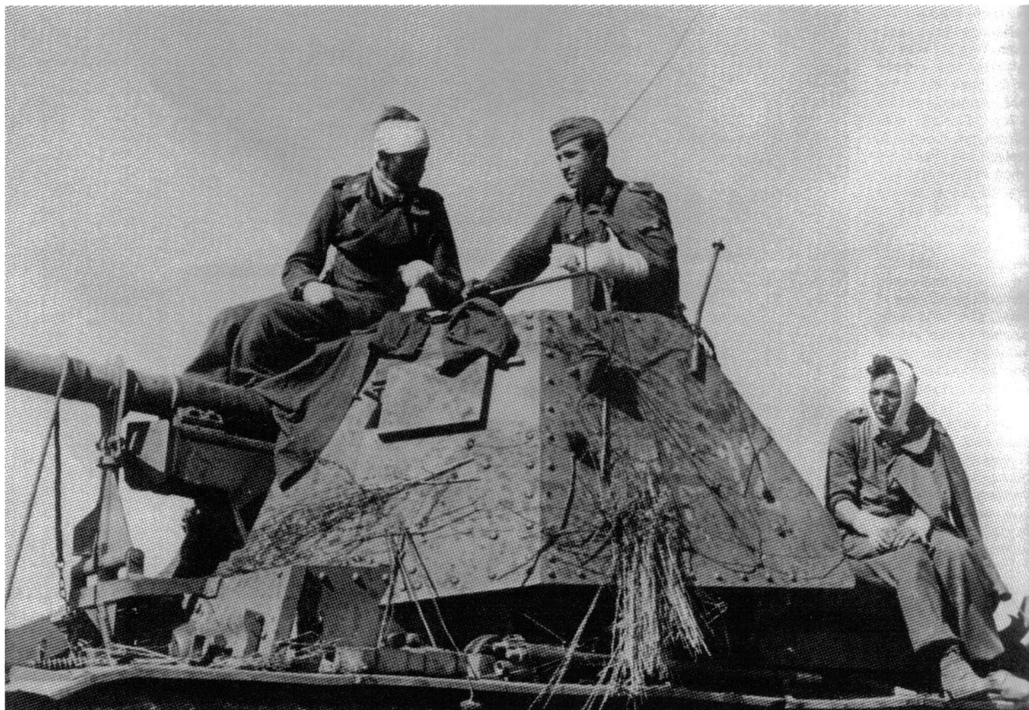
Alive, but a little worse for wear, the crew of this 7.5cm PaK40/3 auf Panzerkampfwagen 38(t) Marder III Ausf.H self-propelled anti-tank gun are back on board and ready for the next battle, late September 1943. Just visible under the foliage is a white outline black national cross and a white two digit tactical number '12'. Built on the chassis of the Czech Pz.Kpfw. 38(t), the Marder III series of self-propelled anti-tank guns were an interim solution while purpose built tank destroyers such as the Jagdpanzer IV and Jagdpanther were being developed. They served with the Panzer-Divisions, Panzer-Grenadier-Divisions and some Infantry Divisions in the Panzerjäger Abteilungen and also with independent Panzerjäger units.
