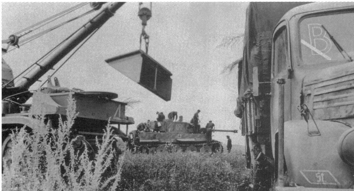
Two photographs of Tiger '122' from s.Pz.Abt.503 in the middle of August 1943. In the lower photo, the crew and mechanics are taking a break. The tank displays many signs of combat it has seen; missing mudguards and tools, a missing smoke candle discharger, a damaged roadwheel and a bent antenna. The missing mudguards also provide some insight on how the camouflage paint has been applied.
