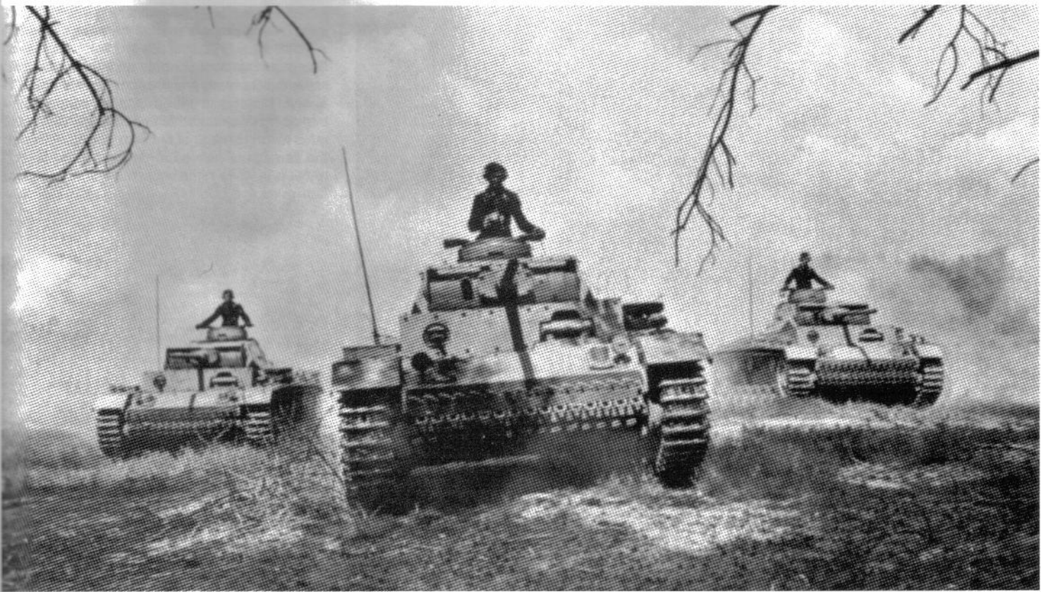
Three Pz.Kpfw.III Ausf.L in what appears to be a propaganda photo of charging Panzers. The 5cm KwK39 L/60 gun was introduced in the Pz.Kpfw.III Ausf.J in December 1941 and continued with the Ausf.L until December 1942. Their armored protection was upgraded by the addition of 20mm spaced armor plates on the upper hull and mantlet, however, due to the late delivery of a new torsion bar counter-balance for the main gun, many did not receive the mantlet armor.
