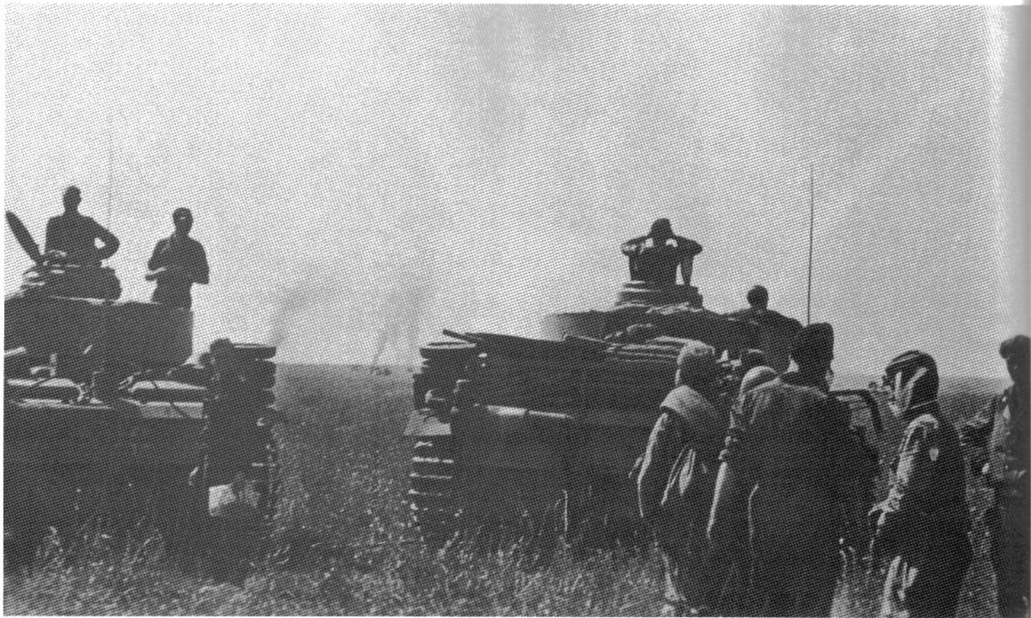
Two command Pz.Kpfw.III observe the battle in the distance, July 1943. The vehicle on the left is a Pz.Kpfw.III Ausf.K, based on the Pz.Kpfw.III Ausf.M, but fitted with a modified Pz.Kpfw.IV turret equipped with a 5cm KwK39 L/60 gun. It has an unusual two digit tactical number, '22', painted in white outline on the rear of the turret schürzen. A star antenna is mounted in the center of the engine deck. On the right is a standard Pz.Kpfw.III Ausf.M being used as a staff vehicle. Note the deep wading exhaust on both.
