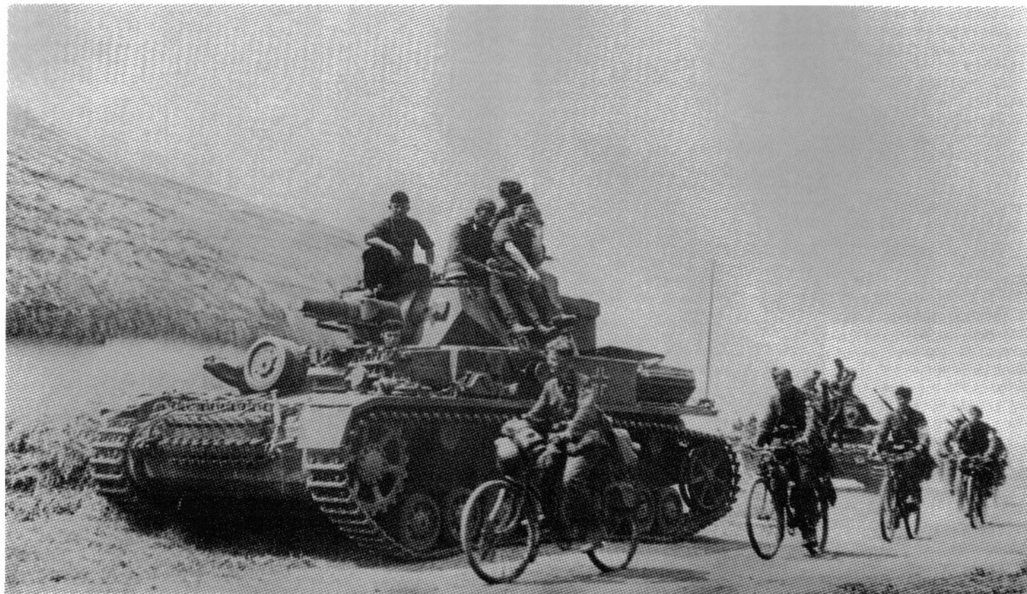
A Pz.Kpfw.IV Ausf.F1 is passed by a group of infantry equipped with bicycles. Armed with the 7.5cm KwK37 L/24, it was only capable of dealing with the Soviet KV-1 and T-34 at short ranges. The introduction of the Pz.Kpfw.IV Ausf.F2, seen behind, armed with the 7.5cm KwK40 L/43, finally gave the Germans a technical superiority. Interestingly, the antenna has been field mounted on the rear of the left mudguard.
