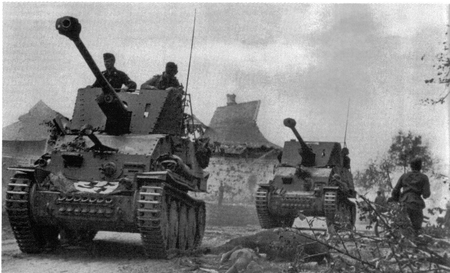
Two Panzerjäger 38(t) für 7.62cm PaK36(r) Marder III tank destroyers. Over 350 of these vehicles were built from April to October 1942 and served mainly with Panzerjäger units in Russia. It was a simple adaptation of the obsolete Pz.Kpfw.38(t) tank chassis and captured stocks of the Soviet 7.62cm Field Gun Model 1936. The barrel was rechambered to accept a 7.5cm PaK40 cartridge. Note the German national flag draped over the front of the leading vehicle for air recognition.
