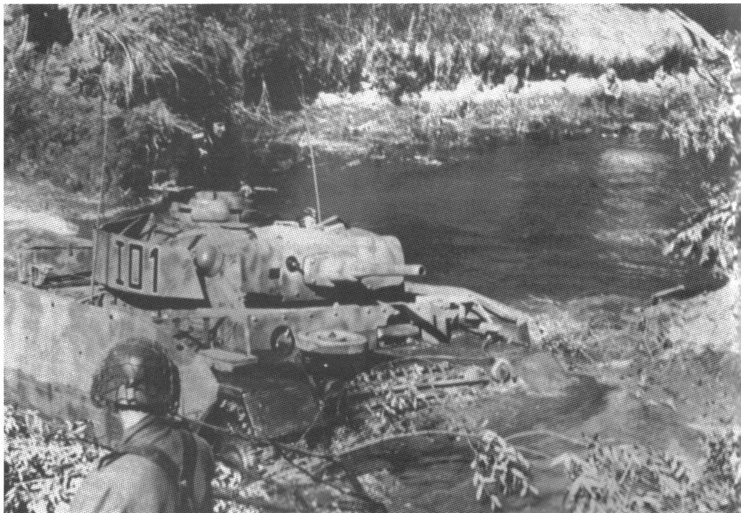
A Pz.Bef.Wg.III Ausf.J assigned to the I.Bataillon commander, Pz.Rgt.25, crosses a small stream near Kursk in July 1943. It has been fitted with the additional 20mm spaced armor plates to the front of the hull and gun mantlet as well as a complete set of schürzen around the turret and sides of the hull. A textbook camouflage pattern of light green and brown has been sprayed over the dark sand base color and new tactical markings, '102', have been painted in black with a white outline on the turret schürzen. The new black inverted 'T' insignia of 7.Panzer-Division is visible on the front plate beside the driver's visor.
