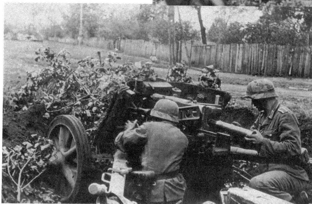
Few Soviet tanks were safe at ranges below 500m when they appeared in the sights of the 5cm PaK38, especially when using the powerful, but uncommon, Pzgr.Patr.40, capable of penetrating 116mm of armor plate at that distance. This was drastically reduced to 72mm at a range of 1000m. Here we can see one of these guns in action on the outskirts of a Russian village near Achtyrka. As well as camouflaging their gun, the crew have also camouflaged their helmets, probably with mud.
