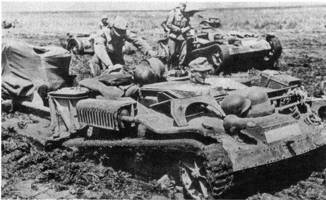
A pair of Renault UE tractors plow their way across the muddy Russian steppe after a rain storm in the spring of 1942. They normally had a crew of two men and had a large, open tray in the rear for carrying a load. Officially incorporated into the Wehrmacht, they were assigned a standard license number that would have been painted in the white rectangle on the front of the hull. It would appear that these two have not yet had their numbers assigned.
