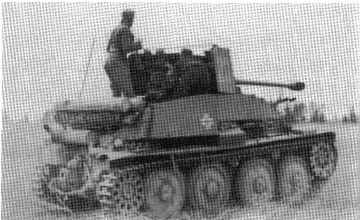
Another photo of a Marder III in action during the summer of 1942. It is obvious the space within the crew compartment was very limited and only provided partial protection against enemy small arms fire and shell splinters.
