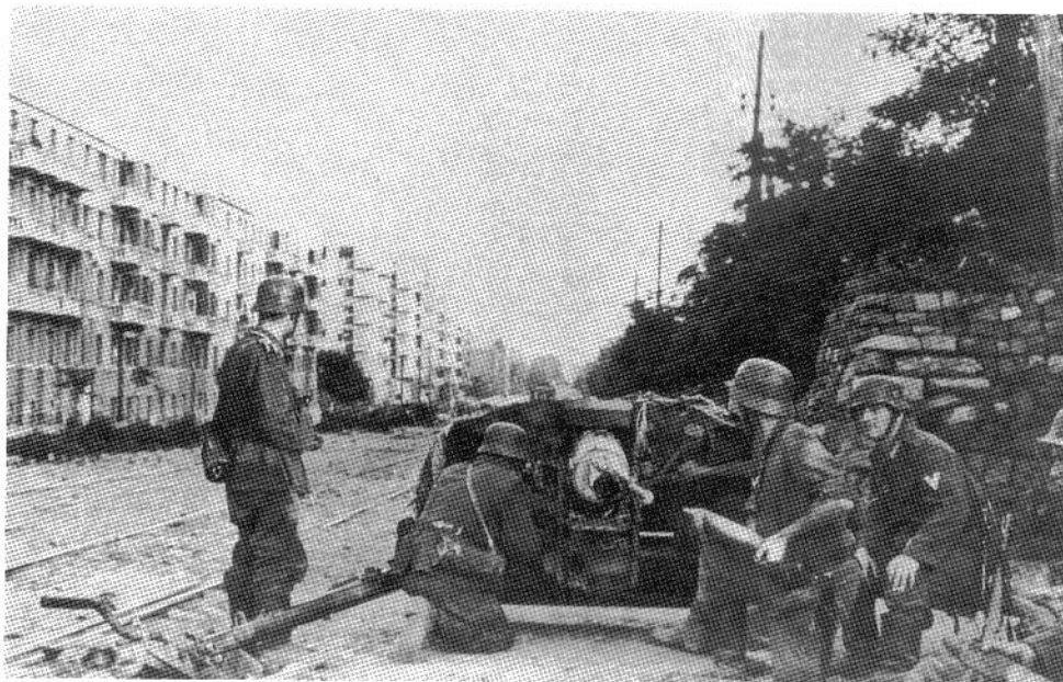
A 7.5cm PaK97/38 anti-tank gun and its six-man crew guard a street in the newly captured city of Rostov on Don in the middle of July, 1942. The gun was introduced as an interim measure when the Germans first encountered the new KV-1 and T-34 tanks in Russia, by adapting the barrels from captured French Model 1897 field guns to the carriage of the 5cm PaK38. Although the carriage is painted in dark gray, the breech remains in white in the same manner as standard tank guns.
