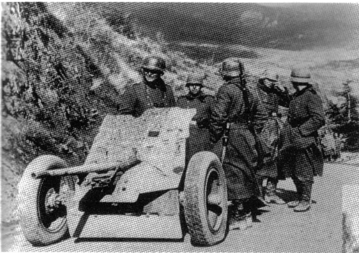
A mud spattered 3.7cm PaK35/36 anti-tank gun blocks a road in the Crimean Peninsula in November, 1941. This gun was often used in an infantry support role as it was incapable of dealing with the heavier tanks of the Red Army now being encountered in greater numbers.
