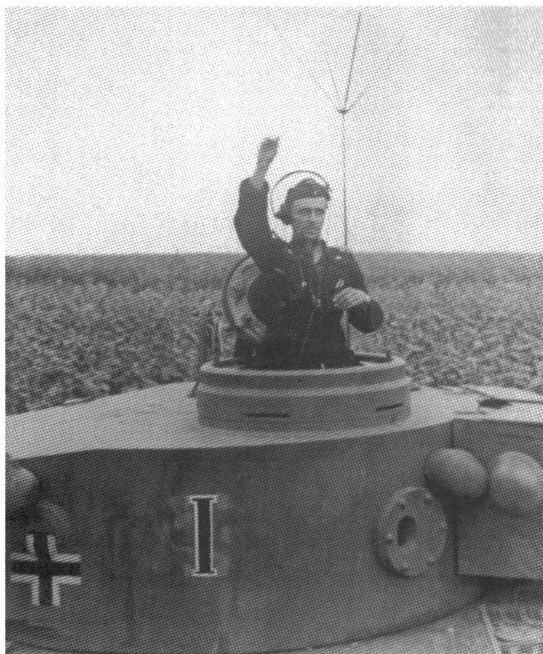
An Oberleutnant from the battalion staff signals to a comrade from the turret of a Panzerbefehlswagen Tiger in August 1943. Very few Befehlswagen Tigers were built and of those, 18 were converted back to standard gun tanks in November 1943. They were equipped with additional long range radios, a Fu 8 with a star antenna fitted to the right side of the engine deck, or a Fu 7 with a 1.4m antenna on the left side of the engine deck plus the standard Fu 5 with the 2m rod antenna mounted on the turret roof. The tactical marking 'I', which is painted black with a white outline, indicates this is the tank assigned to the battalion commander of S.Pz.Abt.503.
