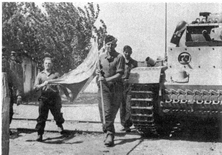
An early Pz.Kpfw.III Ausf.J with the 5cm KwK L/42 gun which has been backfitted with a 20mm spaced armor plate on the front of the upper hull and brackets for a 20mm plate on the mantlet. The tactical sign for 13.Panzer-Division is clearly seen painted in yellow on the side of the hull. Of special interest is the installation of the S-Minenwerfer on the mudguard otherwise only seen on the Tiger I. This photo was taken in the Kuban during the summer of 1942.
